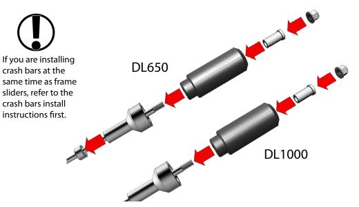
Assemble as shown. Tighten the M12 locking nut with an 18mm socket so that just one thread is showing past the top of the nut. Use the spacers shown above for the DL650. Spacers not needed for the DL1000.
