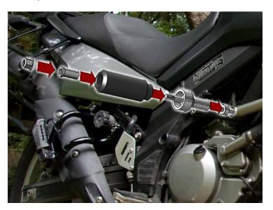
Now assemble the second side of the frame sliders as shown. Using (2) 18mm sockets w/extensions, tighten both sides down. Use the torque wrench to tighten both sides to 60Nm. (spacer not needed for the DL1000)
