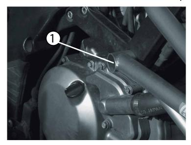
Using (2) 17mm sockets w/ratchets, remove the AltRider provided through bolt from the Crash Bars' frame mount.
