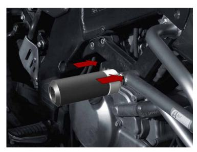
Insert the assembly through the crash bars' frame mount as shown above. Push this whole assembly through until the frame slider is seated firmly in the crash bars.
